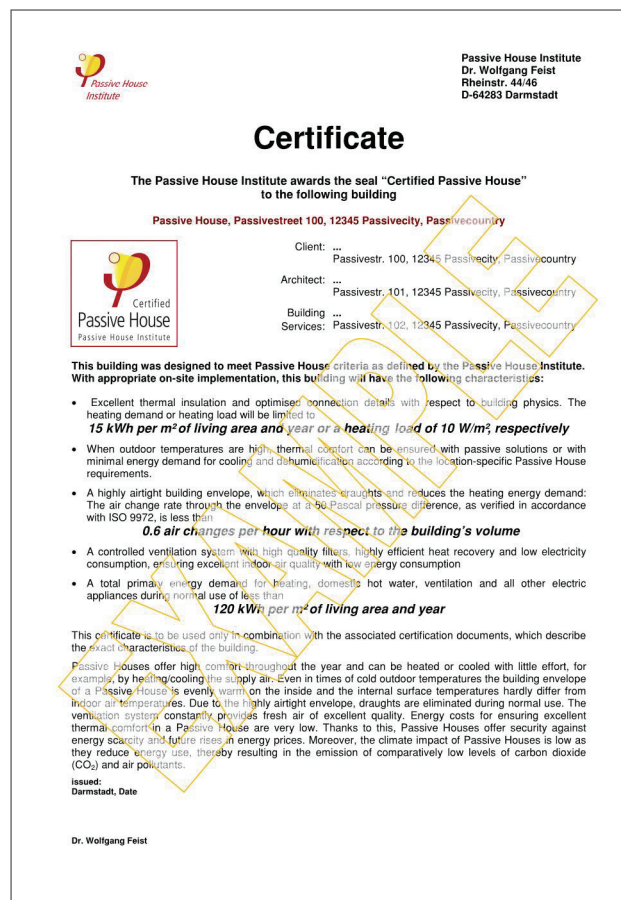
24.09 Passivhaus Certificate. Each house is individually tested and assessed to ensure that it meets the Passivhaus standard and a certificate is issued by the Passivhaus Institute in Germany.
