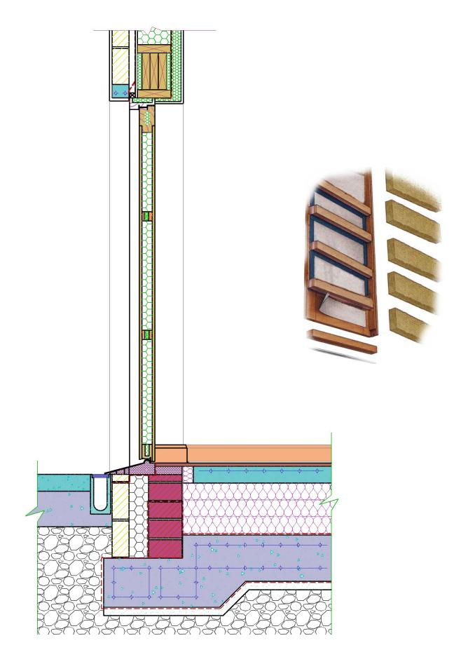
(i) Best practice details for threshold, floor, door and wall- foundation not required such as
